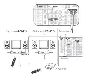
Different sources can be playing in three rooms at the same time or, depending on your needs, the same source can also be used. The main and sub rooms have independent power (the main room power can be off while one (or both) of the sub rooms is on) and the sub rooms can be controlled by the remote or front panel controls. However, you may need to specify the volume settings in *Multi-Room setup* on page 65.
